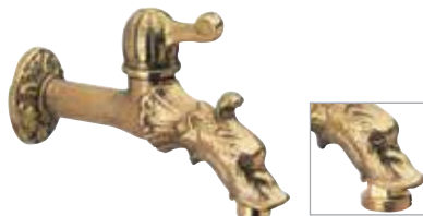
202 LE € 29,40 Rubinetto curvo da giardino in ottone giallo trattato, 1/2 a leva, con rosetta pesante, aeratore e riduzione 3/4 per portagomma. Plain-end garden bibcock, heavy duty, in treated yellow brass, 1/2, lever type, with heavy flange, aerator and 3/4 reduction for hose connection.
